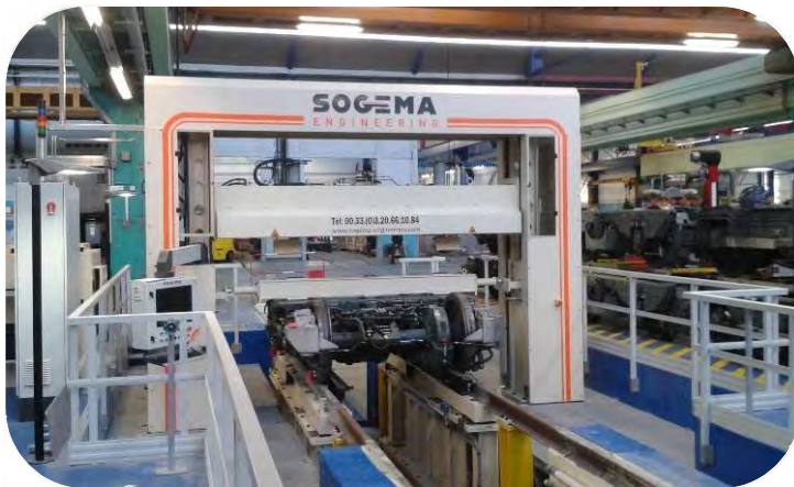
Bogie load testing press with inspection pit
