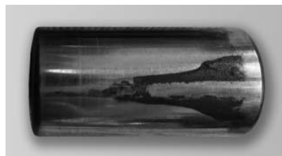
False brinelling on rollers
