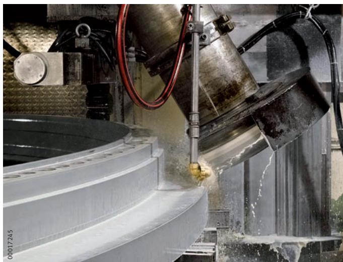
Figure 3 Regrinding of large size bearing ring
