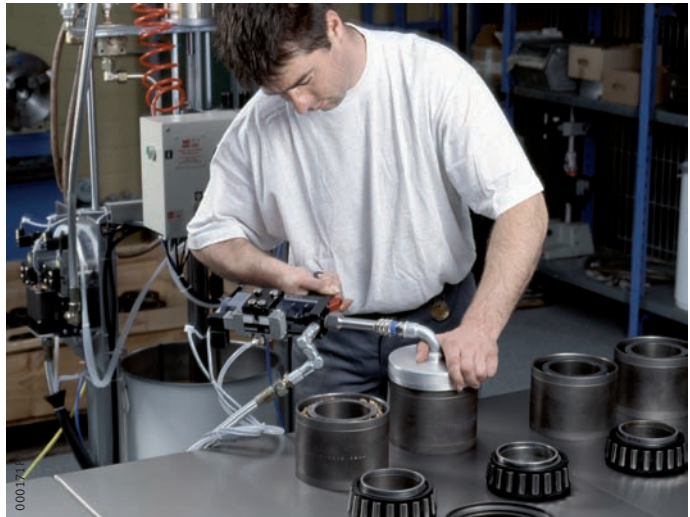
Figure 1 Greasing of TAROL units
