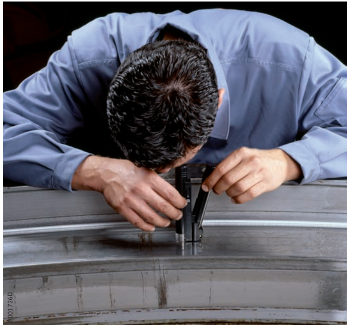
Figure 1 Examination of the raceways on a bearing for a tunnel boring machine
